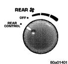
Rotating this knob left to the "REAR CONTROL" position allows the passengers in the second and third row seats to control the blower speed and temperature by means of the rear control located in the rear of the center floor console as described under "Rear Zone Control." Rotating this knob
